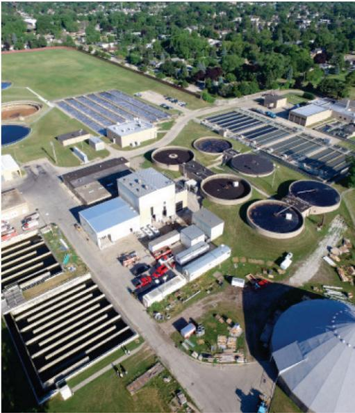
In response to rising landfill disposal fees and energy costs, the Kenosha Water Utility (KWU) redesigned its solids management process to reduce reliance on purchased energy and landfilling the biosolids. Two combined heat and power (CHP) generators were installed to use the biogas as a fuel source. The CHP units are each capable of producing 330 kW of electrical energy and 422 kW of thermal energy.
